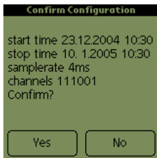
Figure 12: confirmation dialog for programming parameters in this example the start date and time are 2004, December 23 at 10:30, the stop date and time are 2005, January 10 at 10:30, the samplerate is 4 milliseconds and the channels 1, 2, 3 and 6 are active
